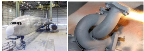
Figure-5: Thermal spray coating application in aerospace and in automotive (to coat exhaust system) industry
