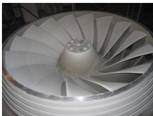
Figure-7: Turbine blade sprayed with ZrO_2 coating using Plasma Spray
