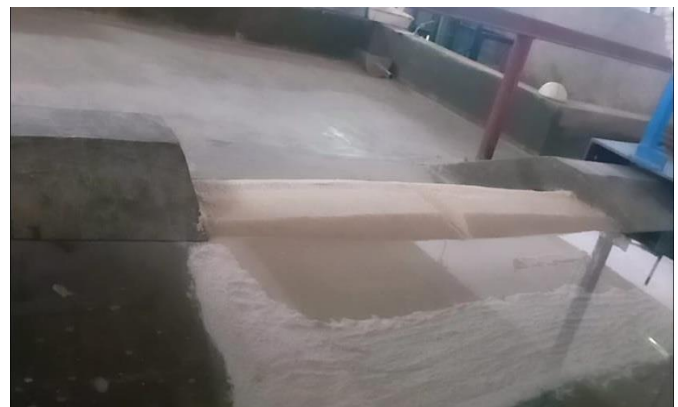
Fig – 2 Levee breach during experiment
