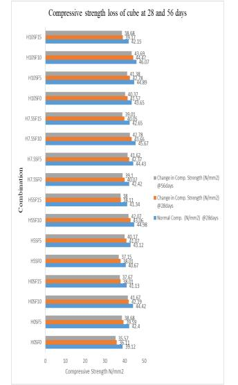
Figure 5 Loss of Compressive Strength N/mm<sup>2</sup> at 28 and 56 days
