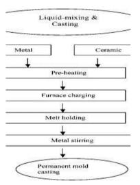
Fig5.4: Steps in stir casting
