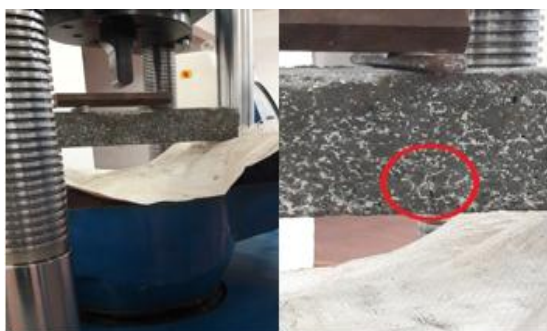
Fig. 4. Flexural strength test on beam
