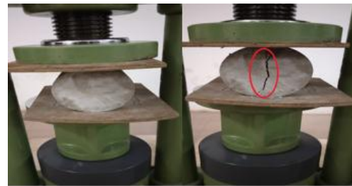
Fig. 3. Split tensile test on cylinder
