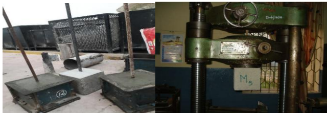
Fig. 5. Pullout test of specimens
