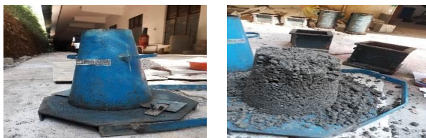
Fig. 1. Slump cone apparatus and obtained slump
