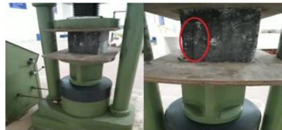
Fig. 2. Compression test on cube
