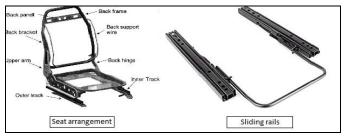
Fig -2.4: Four wheeler seat structure
