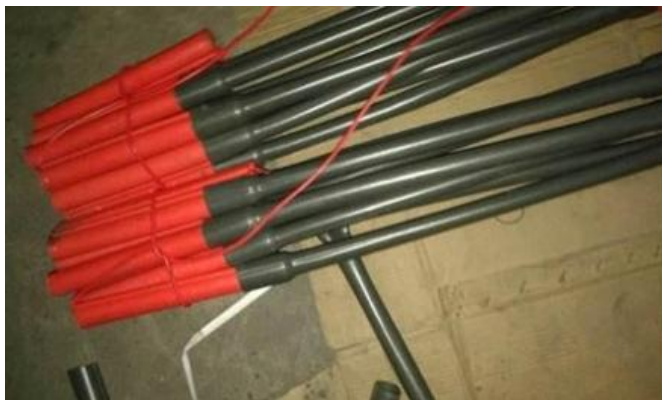
Fig. 3.6. Spacers Connected with an Explosive Cartridge.
