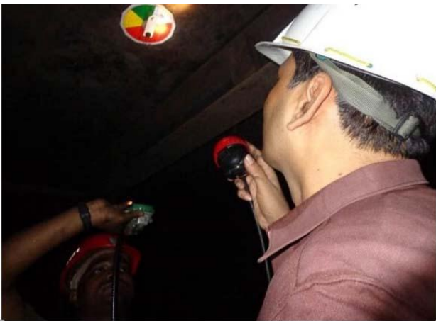
Fig.3.11. In-situ measurement of convergence.
