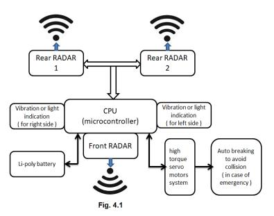
The Fig. 4.1 Shows the block diagram of the CAS system for bikes. The function of each block is as follows:
