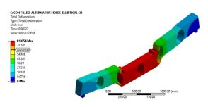
c) Concrete in-filled beam with alternative holes
