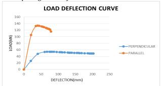
Fig.8 Load Deflection curve of diaphragms
