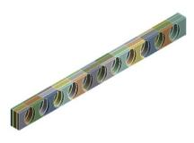
b) Concrete filled castellated beam with holes
