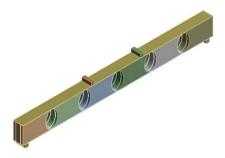
c) Concrete filled castellated beam with alternate holes
