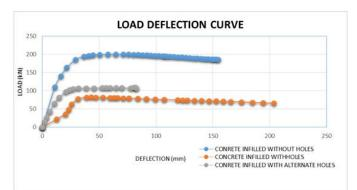
Fig. 9 Load Deflection curve of concrete in-filled beam
