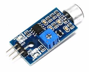
Fig4 LM393 sound sensor module
