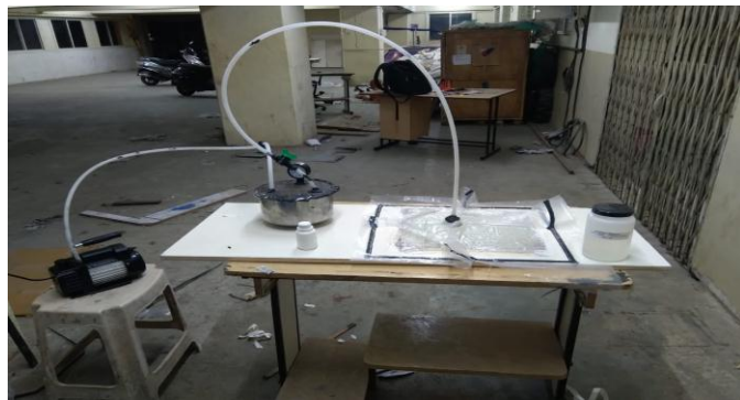
Fig 1 : Vacuum bagging process
