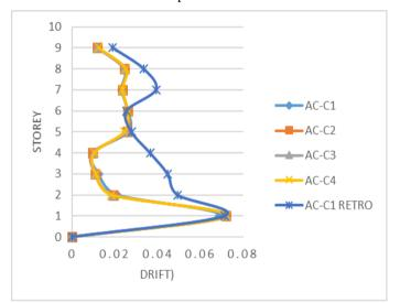
Fig 6: Graph with storey vs driftt across the slope
