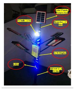
Fig. 6 Structure of Solar Tree
