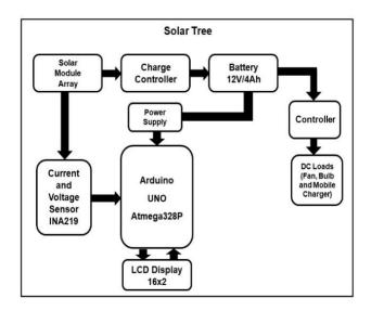
Fig. 5 Block Diagram of Solar Tree
