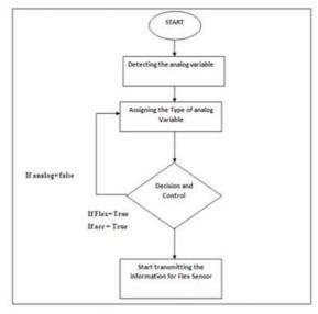
basic flow diagram for transmitter
