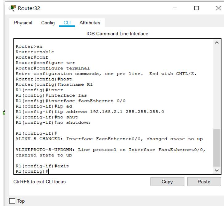
Fig 3.4: Different interfaces of Cisco Router. Fig 3.5: Configuration of IP address to interface
