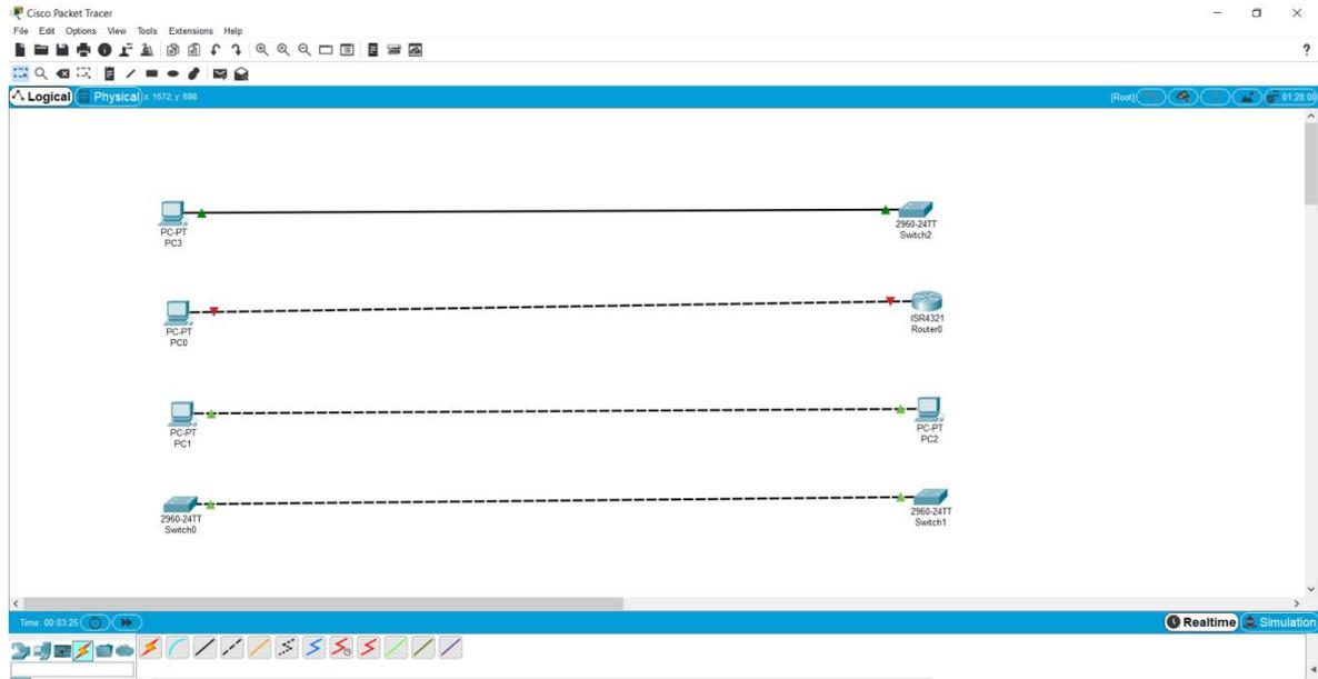
Fig 2.2: Workspace of Cisco Packet Tracer: Cables used for connecting different devices
