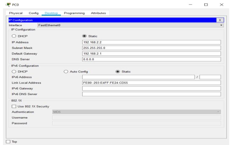
Fig 3.2: IPV4 configuration-assigning IP address
