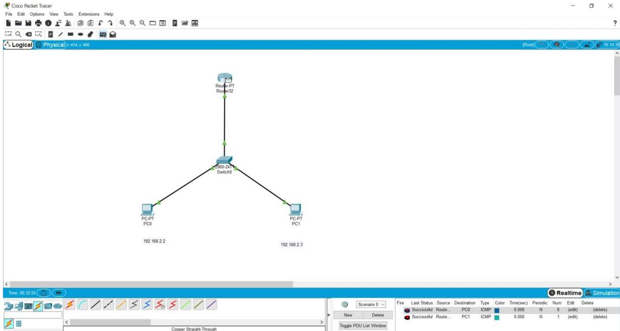
Fig 3.3: Packet transformation successful from router to PC, PC to router through switch
