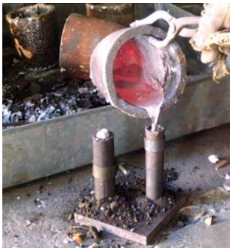
Fig. 3. Pouring of molten metal into the cast iron molds
