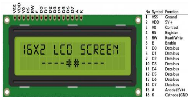
Figure 5: 16X2 LCD Screen
