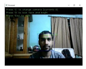
This face recognition algorithm is applied to the frame in the video and outputs a bounding box for each face it detects. To maintain consistency across frames, if there is no face detected in frame ,the face from the previous frame is used, if there is multiple face detected in the frame, the face that is nearest to that frame is used.
