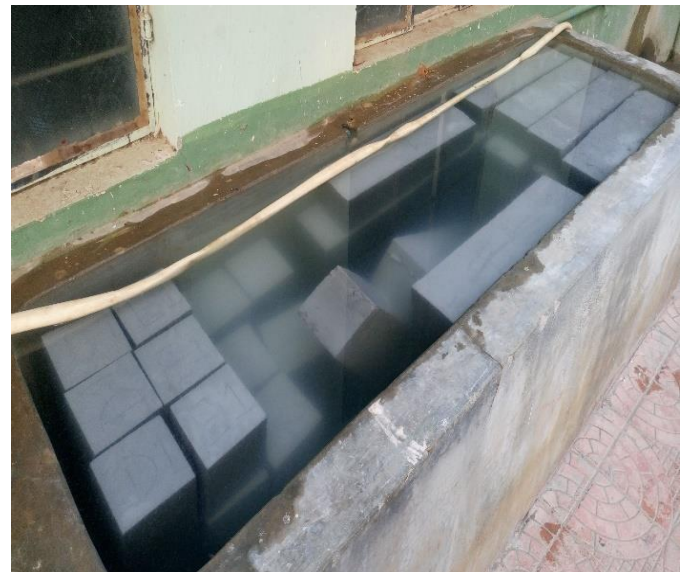
Fig -2: Curing of Cubes and Beams
