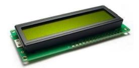
Fig -2: Liquid Crystal Display
