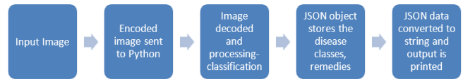
Fig -3: Steps taken in methodology at the client end of our demo application
