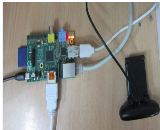
Fig - 1: Connection of USB Camera with Raspberry Pi
