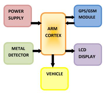
These are main components present in designing landmine detection robot:
