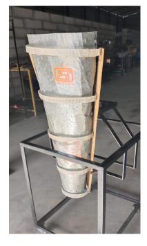
Tin sheet is used for making this structure because it is cheap and easy to bend and mounting is also easy on this tin sheet.
