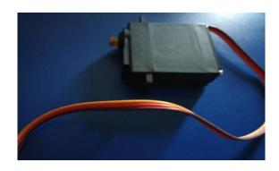
A Servo motor is a rotary actuator or linear actuator which provides precise control for the angular motion and linear motion.
