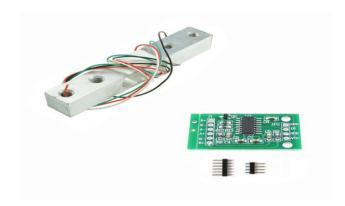
Load cell is a kind of transducer which converts the load, force or weight into an electronic signal. It contains a strain gauge. Strain gauge is basically an elastic material, so when force or load act on it, it deflects, so the resistance change within the strain gauge, so if we supply voltage the output voltage gets vary this variation is used for measuring the load or force acting on it.
