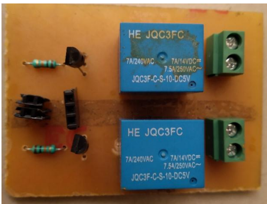
Fig -7: Relay circuit.
