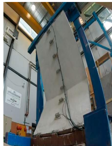
Fig-2: Extreme deformations of single sided wall [4]
