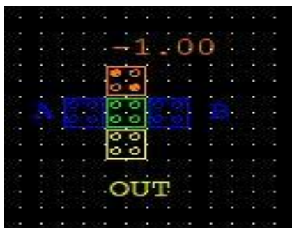
Fig -6: AND Gate Layout
