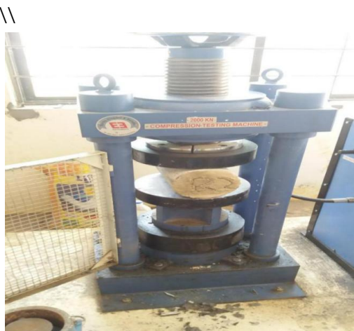
Fig. 2: testing of split tensile strength
