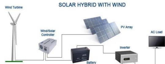
Fig.4.2 block diagram of hybrid power generation system
