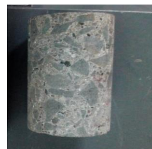
Fig -2: Core sample of Beam 01
