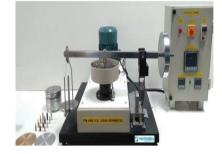
Figure 4: Pin-on-Disc Wear Machine
