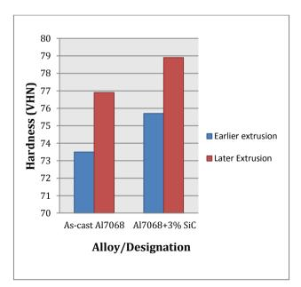
Figure 5: Hardness test values of A7068 alloy and its composites earlier and later extrusion.
