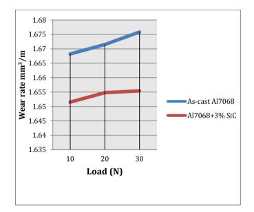
Figure 9: Wear rate test values of A7068 alloy and its composites earlier extrusion.
