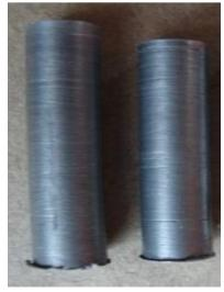
**Figure 11: Wear Tested Specimens**
