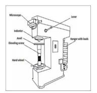
**Figure 3: Vicker Hardness Tester**
