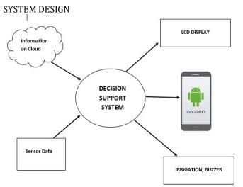
The picture above shows the system architecture. The arrows in the diagram shows the connectivity between the components. The information which is on the cloud and sensor data acts as input to the system and the output required is fetched through LCD display or any android application and any activities like buzzer sound, irrigation etc. The DSS includes a controller which is a circuit based and is programmed to action as per sensor data.
