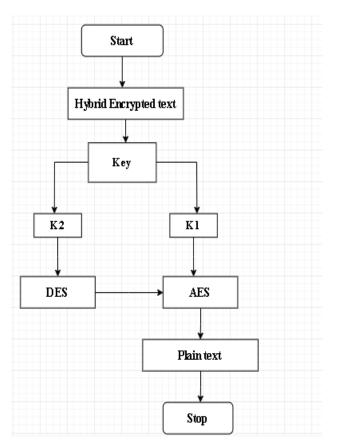
**Fig-2: Flow chart of Decryption Process**
