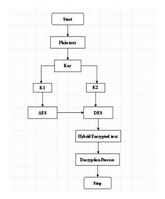
**Fig-1: Flow chart of Encryption Process**
