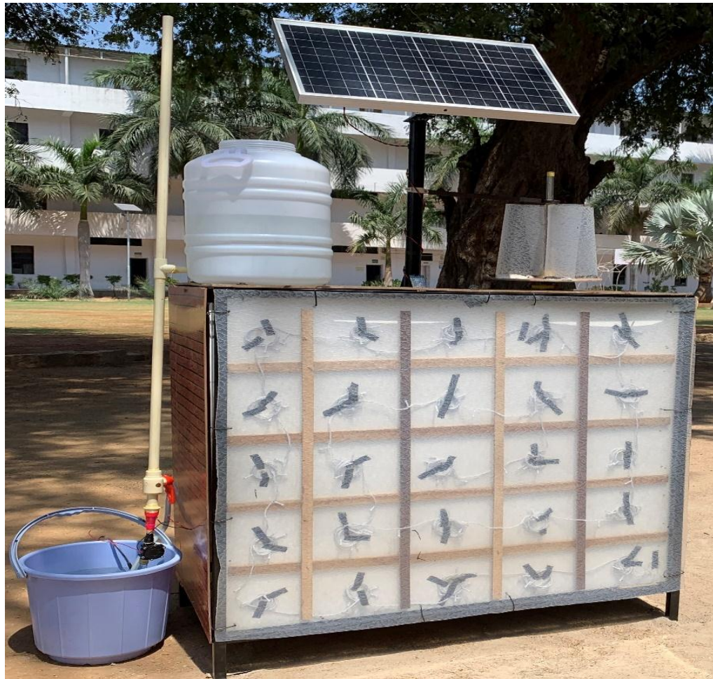
FIGURE 1: HYBRID POWER GENERATION SYSTEM.
