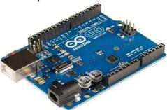
and analog input/output (I/O) pins that may be interfaced to various expansion boards ('shields') or breadboards (For prototyping) and other circuits. The microcontrollers can be programmed using C and C++ programming languages. The Arduino project provides an integrated development environment (IDE) based on the Processing language project.
