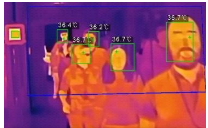
Fig -3: Temperature checking system
