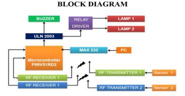
Fig -1: Block diagram of proposed system
