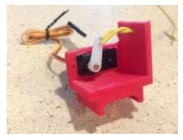
Seed dropping box is mounted on the bottom of the drones. The box contains a servo mechanism and the seeds of the selected plants inside it. The servo is to be connected with the receiver and when the signal is given by the transmitter the servo will be turned on the seed will get drop, how much times the switch and the dropping hatch will on the number of seeds for dropping directly depend on it. This is how the seeds dropping mechanism will going to be work.
