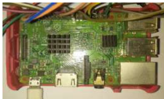
Fig -3: Raspberry Pi 3 with all sensors connected through GPIO
