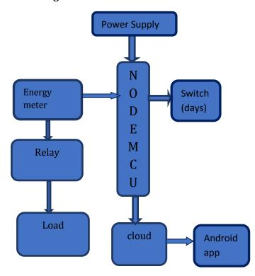
Fig: 1 Block Diagram of Electricty Energy Meter
