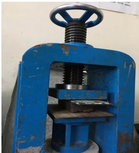
Fig -1: Experimental Setup for Compression test
