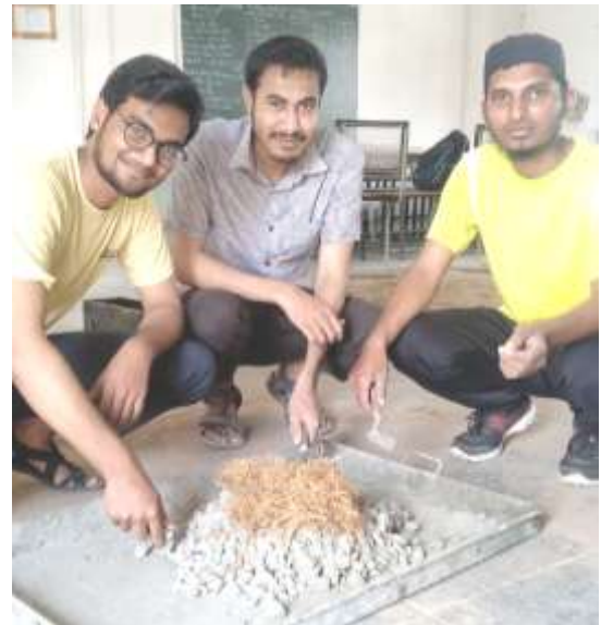
Fig -4: Mixing of Concrete with Fibers
