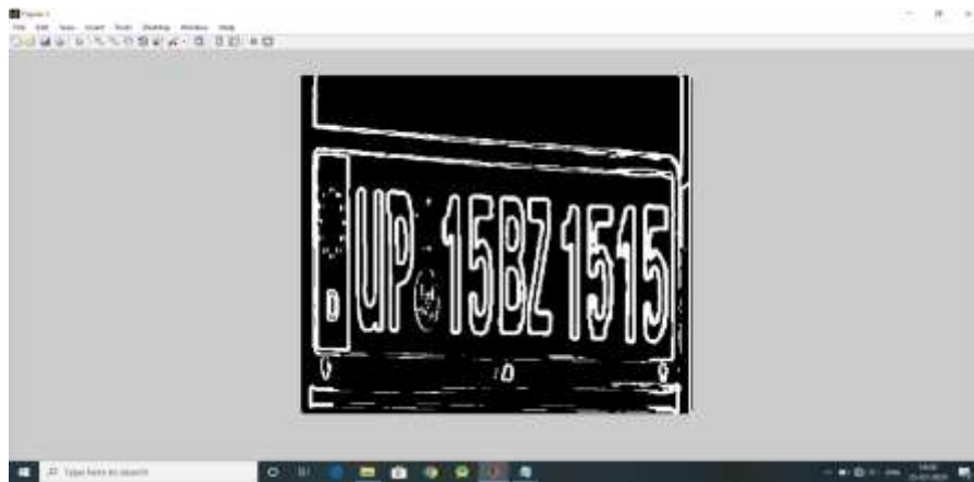
Figure: 2.5 – Image after applying SOBEL Algorithm for filling holes:
