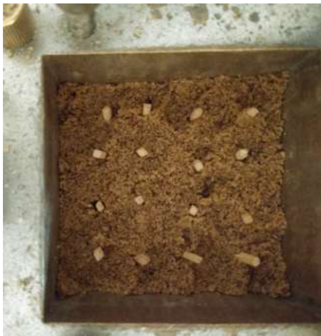
Fig -7: Alignment of wood in vertical direction with 12 mm spacing
