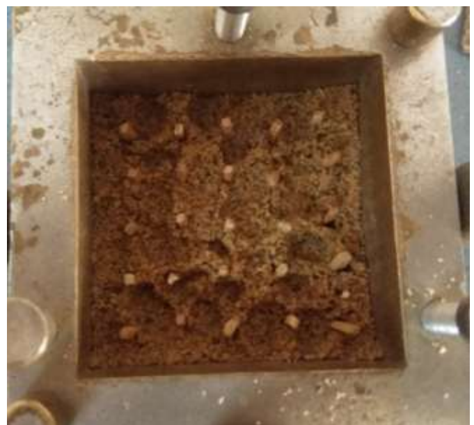
Fig -8: Alignment of wood in vertical direction with 8 mm spacing
