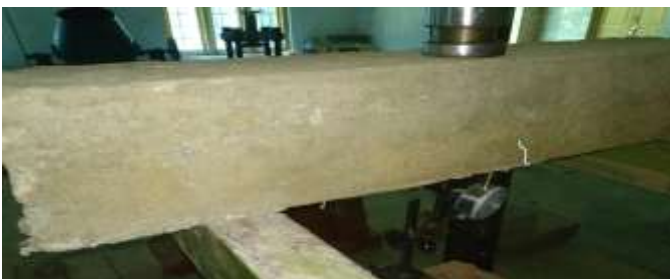
Figure 7: Experimental set up of beam in one point loading
