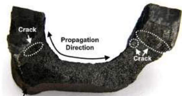
Fig -2: Crack development on runner
