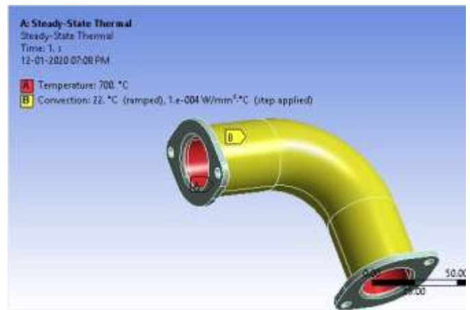
Fig -4: Thermal boundary conditions
