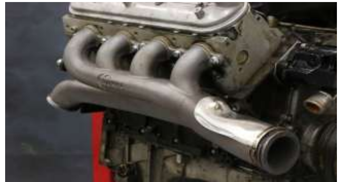
Fig -1: Engine - exhaust manifold assembly
