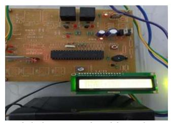
Npk fertilizer ratio is obtained by interfacing Pic microcontroller with temperature, humidity and moisture sensor using MpLab IDE software. The program is burned in microcontroller using pic kit3.
