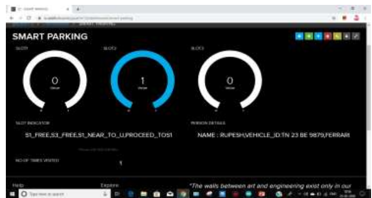
Figure 3. The slot 2 is filled and for the next user the web page displays S1 and S3 are free but S1 is near to you.
