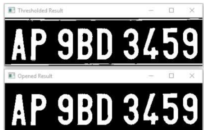
Fig 3.2: Thresholded Result of the image
