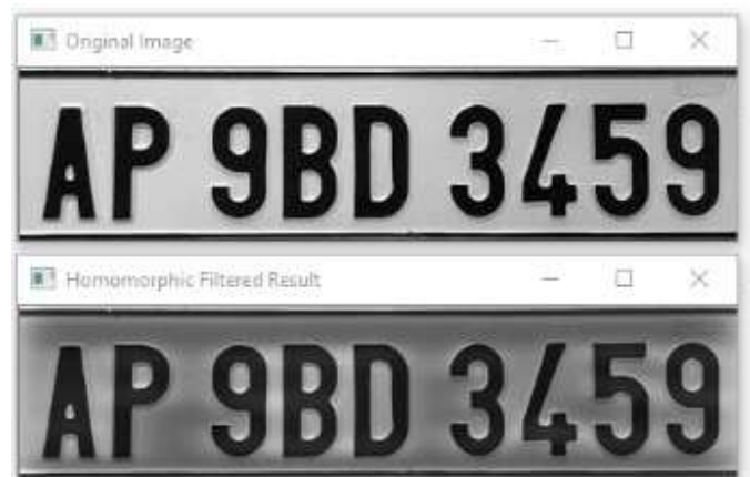
Fig 3.1: Applying Homomorphic Filter
