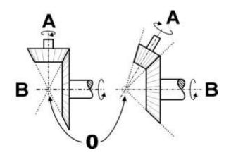
Bevel gears are most often mounted on shafts then they are 90 degrees apart, but can be designed to work at other angles .The pitch surface of bevel gears is a cone.
