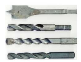
Drill bit are used to cutting the tool and it is used to remove the metal to create holes, almost of circular cross-section. Drill bit come in many sizes and shapes and can create different kinds of holes in different type of material. In order to create holes drill bit are usually attached to a drill, which power them to cut through the work piece by an rotation. The drill bit fixed on the upper end of the shank
